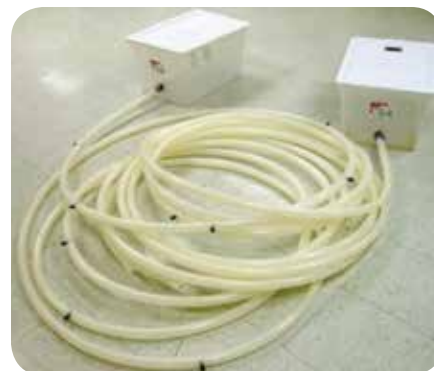
FIGURE 1 Testing apparatus for verifying VCI diffusion with no air movement.
