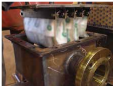
FIGURE 7 An example of a plenum that could be installed to introduce VCI A to a sprinkler system.
